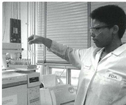
An FDA chemist uses a device set to the same temperature as an activated e-cigarette. This helps determine what might be inhaled by users of these products.
